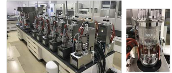
30 L fed-batch culture system with exhaust gas analyzer and autosampler
