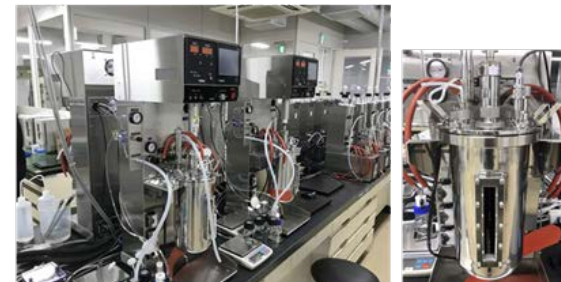
5 L×4 fed-batch culture system with exhaust gas analyzer and autosampler
