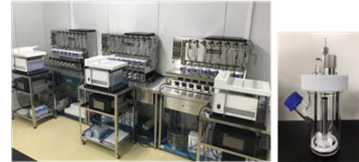
5 L×4 fed-batch culture system with exhaust gas analyzer and autosampler
